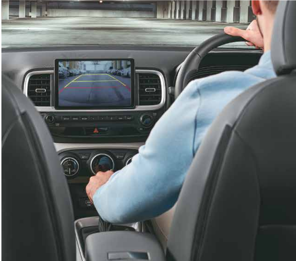
Rear parking assist camera with dynamic guidelines
