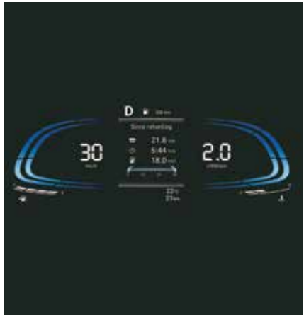
Digital cluster with colour TFT MID
